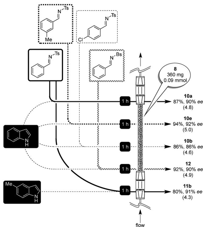
**Figure 5.** Enantioselective continuous-flow production of a library of 3-indolylmethanamines. Productivities [mmol h<sup>-1</sup> g<sub>resin</sub><sup>-1</sup>] are shown in parentheses.
