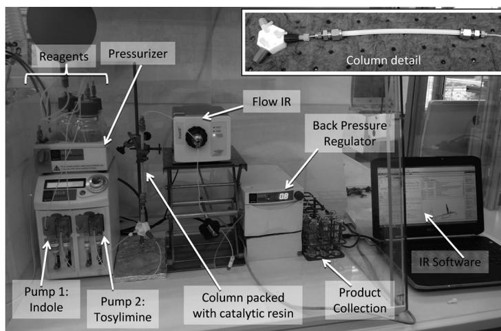
Figure 3. Continuous-flow setup. Inset: column.
