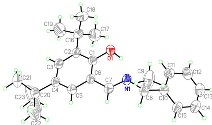
**Fig. 5.** ORTEP diagram of (*R*)-*N*-(1-phenylethyl)(3,5-di-*tert*-butylsalicylidene) (**HL3\***), showing the atom labeling scheme and 40% thermal ellipsoids. Selected bond lengths (Å) and angles (deg): O(1)-C(1) 1.352(3), N(1)-C(7) 1.265(4), N(1)-C(8) 1.455(4).
