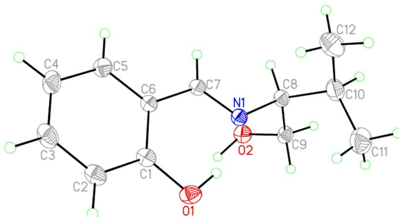
**Fig. 3.** ORTEP diagram of (*R*)-*N*-(1-hydroxymethylisobutyl)salicylidene (**HL1\***), showing the atom labeling scheme and 40% thermal ellipsoids. Selected bond lengths (Å) and angles (deg): O(1)-C(1) 1.354(4), N(1)-C(7) 1.276(3), N(1)-C(8) 1.461(3).
