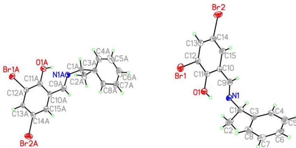
**Fig. 6.** ORTEP diagram of (*R*)-*N*-(1-phenylethyl)(3,5-dibromosalicylidene) (**HL4\***), showing the atom labeling scheme and 40% thermal ellipsoids. Selected bond lengths (Å) and angles (deg): O(1)-C(11) 1.355(10), N(1)-C(1) 1.487(9), N(1)-C(9) 1.242(11), O(1A)-C(11A) 1.330(11), N(1A)-C(1A) 1.477(9), N(1A)-C(9A) 1.269(11).
