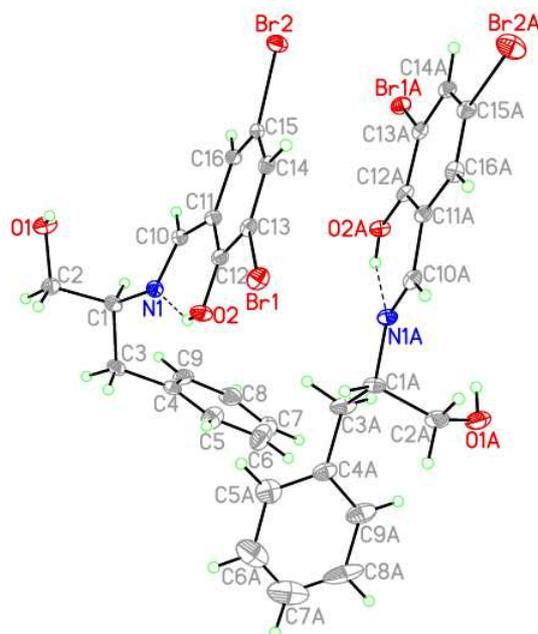
**Fig. 9.** ORTEP diagram of (*S*)-*N*-(1-hydroxymethylphenyl)(3,5-dibromosalicylidene) (**HL7\***), showing the atom labeling scheme and 40% thermal ellipsoids, O–H···N intermolecular hydrogen bonds are depicted as dashed lines. Selected bond lengths (Å) and angles (deg): O(2)-C(12) 1.274(6), N(1)-C(1) 1.463(7), N(1)-C(10) 1.305(6), O(2A)-C(12A) 1.280(6), N(1A)-C(1A) 1.489(7), N(1A)-C(10A) 1.267(7).
