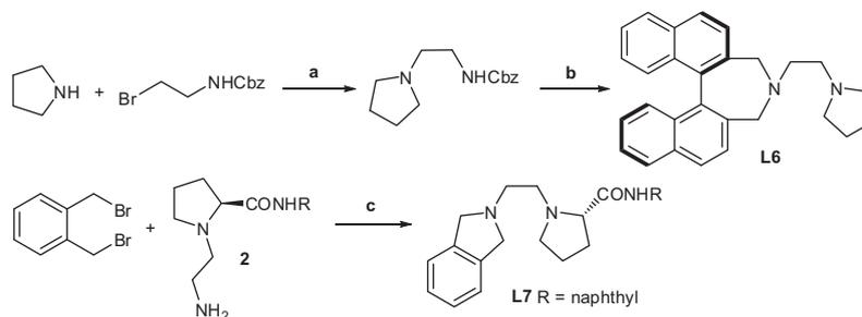
**Scheme 3.** Synthetic routes to comparison ligands **L6** and **L7**: (a)  $K_2CO_3$ ,  $CH_3CN$ , reflux; (b) (i) Pd/C,  $H_2$ , MeOH, rt, (ii) **4**,  $Et_3N$ , DCM, reflux; (c)  $Et_3N$ , DCM, reflux.
