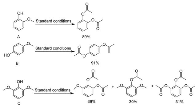
Scheme 2 Reactions with the lignin monomers A, B and C.
