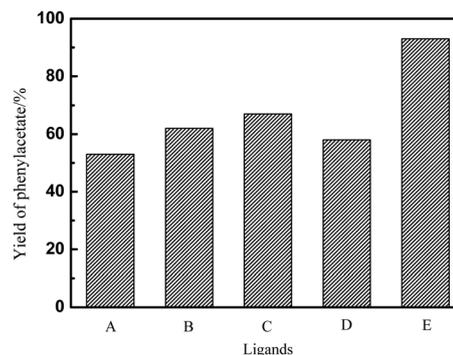
Fig. 1 Yields of phenylacetate catalyzed by IrCl<sub>3</sub> with different ligands. Reaction conditions: 2 mmol anisole, 2 mol% IrCl<sub>3</sub>, 5 mL MeCN, 5 mol% ligand, 3 mmol CH<sub>3</sub>I, 5 bar CO, 180 °C, 20 h. (A) No ligand, (B) 2,4,6-collidine, (C) 1,3-bis(diphenylphosphino)propane, (D) 2,2'-bipyridine, and (E) PPh<sub>3</sub>.
