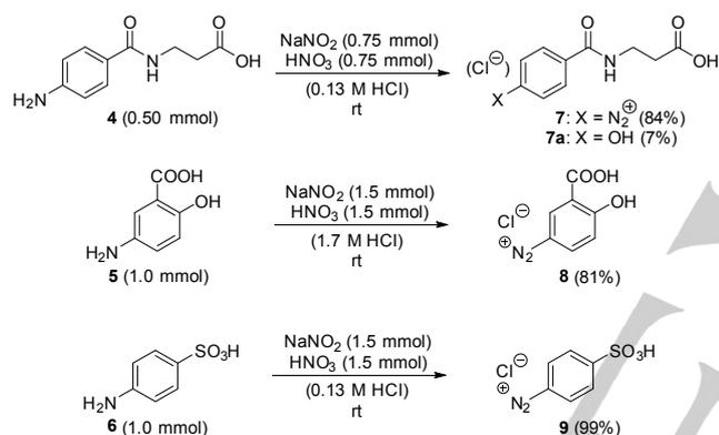
**Scheme 2.** Reaction conditions for diazotization optimized on small scale. Yields determined by <sup>1</sup>H-NMR using maleic acid as internal standard.
