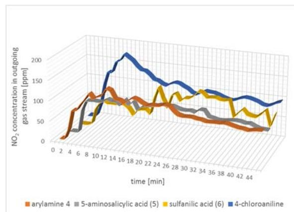
**Figure 2.** Concentrations of nitrogen dioxide in outgoing gas stream after diazotization of arylamines **4-6** and 4-chloroaniline.<sup>[13]</sup>
