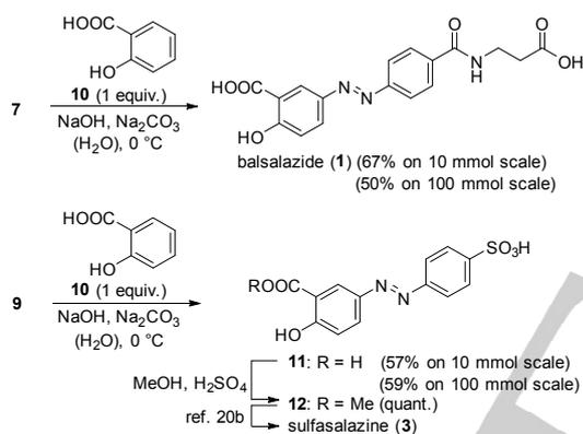
**Scheme 3.** Azo coupling of diazonium salts **7** and **9** – as obtained from wet scrubber – to salicylic acid (**10**) and synthesis of balsalazide (**1**) and sulfasalazine (**3**).
