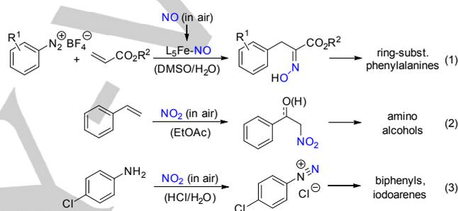
**Scheme 1.** Organic synthesis combined with denitrification: utilization of low-concentrated nitrogen monoxide and nitrogen dioxide.<sup>[12],[13],[17]</sup>
