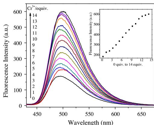
**Figure 1.** Fluorescence spectra of NP-B ( $1 \times 10^{-5}$  M) in THF/ $\text{H}_2\text{O}$  (85/15, v/v) with a buffer solution of 3-(*N*-morpholino) propanesulfonic acid (MOPS, 10 mM, pH = 7.0) in the presence of different concentrations of  $\text{Cr}^{3+}$  (0–14 equiv).  $\lambda_{\text{ex}} = 420$  nm. Inset: fluorescence intensity at 498 nm of NP-B as a function of  $\text{Cr}^{3+}$  concentration.
