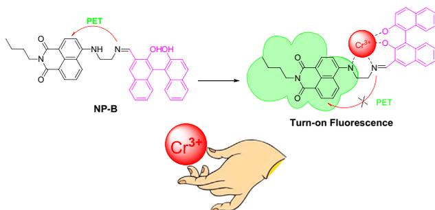
**Scheme 2.** Proposed binding mode of NP-B with  $\text{Cr}^{3+}$ .
