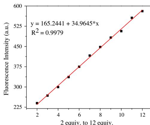
**Figure 2.** Curve of fluorescence intensity at 498 nm of NP-B ( $1 \times 10^{-5}$  M) versus increasing concentrations of  $\text{Cr}^{3+}$  (2–12 equiv).
