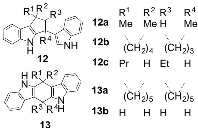
Figure 1. 2:2 Condensation ( $-2\text{H}_2\text{O}$ ) reaction of indole with 2,2-dimethoxypropane
