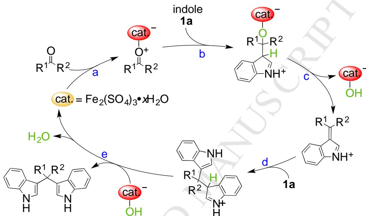
Scheme 1. The proposed reaction mechanism is: (a) Coordination of the carbonyl O atom with an Fe atom, with color change; (b) Nucleophilic attack by an indole-3-C atom at the carbonyl C atom; (c) Elimination of hydrated ferric sulfate hydroxide; (d) Nucleophilic attack by a second indole-3-C atom at the carbonyl C atom; (e) Proton transfer and elimination of water.
