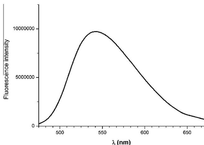
**Figure 2.** Fluorescence emission spectrum of (*R*)-2-amino-4-DMNA-butanoic acid (**2**) in aqueous methanol (1:1) showing a maximum at 543 nm (excitation wavelength was 450 nm).
