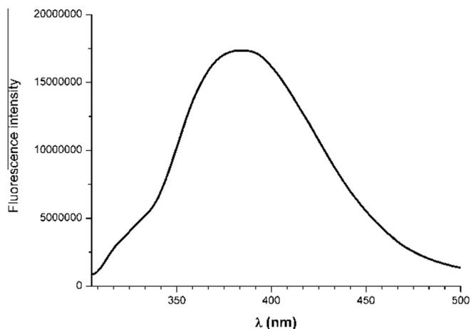
**Figure 1.** Fluorescence emission spectrum of (*R*)-2-amino-3-(*p*-acetamidobiphenyl)propanoic acid (**1**) in aqueous methanol (1:1) showing a maximum at 384 nm (excitation wavelength was 295 nm).
