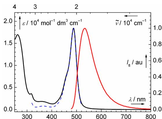
**Figure 1.** Absorption (black solid line), normalized emission (red solid line), and excitation (blue dashed line) spectra of **1** ( $c \approx 1 \times 10^{-5}$  M) in 0.1 M aq phosphate buffer at pH = 7.4.
