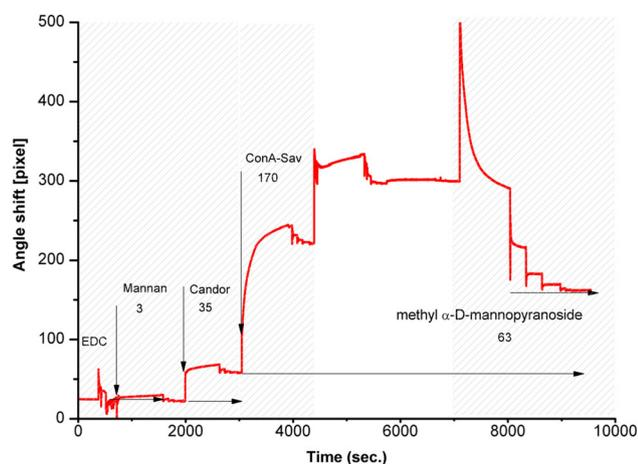
**Figure 6.** SPR-based covalently coupled mannan-ConA-Sav binding on PHCP co-polymer studies: 1. surface activation with EDC; 2. addition of mannan ( $1 \text{ mg mL}^{-1}$ ); 3. blocking step with Candor; 4. addition of ConA-Sav fusion protein. ( $300 \mu\text{g mL}^{-1}$ ); 5. regeneration with 10% methyl  $\alpha$ -D-mannopyranoside.
