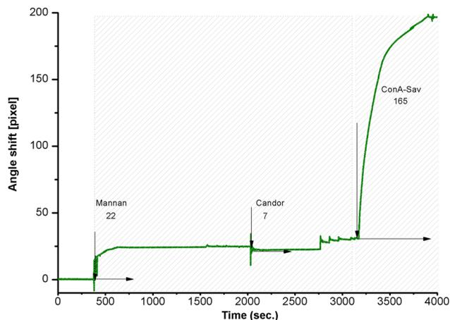
**Figure 7.** SPR-based pyrrole-N-C16 pyrrole co-polymer studies: 1. addition of mannan ( $1 \text{ mg mL}^{-1}$ ); 2. blocking step with Candor; 3. addition of ConA-Sav fusion protein ( $300 \mu\text{g mL}^{-1}$ ).
