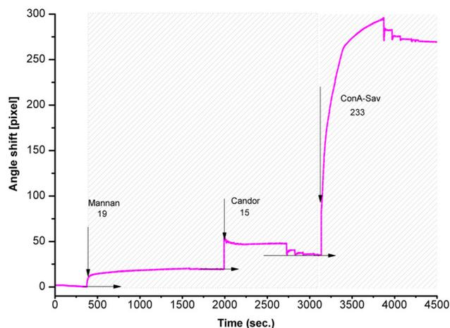
**Figure 8.** SPR-based 4-(1H-pyrrol-1-yl)phenol pyrrole co-polymer studies: 1. addition of mannan ( $1 \text{ mg mL}^{-1}$ ); 2. blocking step with Candor<sup>®</sup>; 3. addition of ConA-Sav fusion protein ( $300 \mu\text{g mL}^{-1}$ ).
