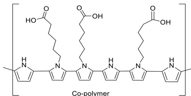
**Figure 4.** Potential structure of a pyrrole/6-(1H-pyrrol-1-yl) hexanoic acid co-polymer (PHCP).
