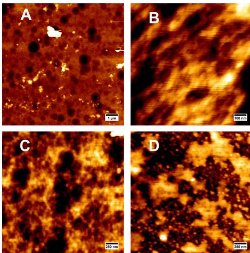
**Figure 9.** AFM height images (cantilever HQ:NSC14AIBS) of modified chips: a) overview of pure gold surface without modification; b) detailed image of pure gold surface without modification indicating smooth surface (roughness 2.56 nm); c) surface modified with pyrrole and mannan; d) surface modified with pyrrol-N-C16 pyrrole co-polymer and mannan + ConA-Sav (increased roughness of mannan and ConA-Sav clusters visible).
