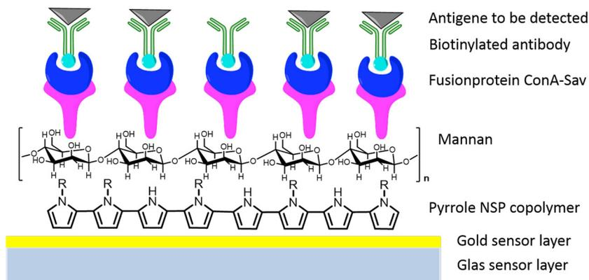
**Figure 1.** Schematic cross section through the layers which are subject of this investigation.
