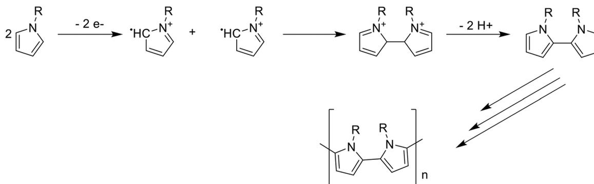
**Figure 3.** General scheme of electro-polymerization of pyrrole building blocks.
