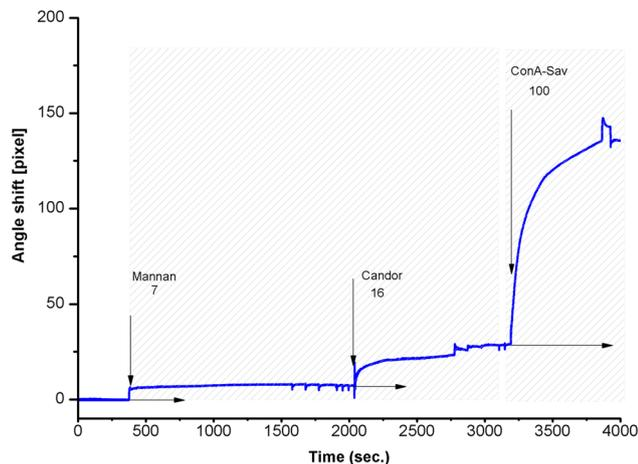
**Figure 5.** SPR-based mannan-ConA-Sav binding on PHCP co-polymer studies: 1. addition of mannan ( $1 \text{ mg mL}^{-1}$ ); 2. blocking step with Candor; 3. addition of ConA-Sav fusion protein ( $300 \mu\text{g mL}^{-1}$ ).
