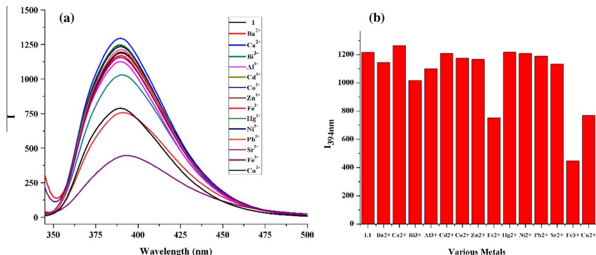
**Figure 2.** (a) Fluorescence responses of **1** ( $1.0 \times 10^{-5}$  mol/L, excitation wavelength = 324 nm) to various metal ions ( $1.0 \times 10^{-5}$  mol/L). (b) Bar representation of fluorescence responses of **1** ( $1.0 \times 10^{-5}$  mol/L, excitation wavelength = 324 nm) to various metal ions ( $1.0 \times 10^{-5}$  mol/L).
