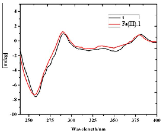
**Figure 3.** CD spectra of **1** and **1** with an equivalent amount of Fe<sup>3+</sup> in acetonitrile ( $c_1 = 1 \times 10^{-5}$  mol/L,  $c_{Fe(III)} = 1 \times 10^{-5}$  mol/L).
