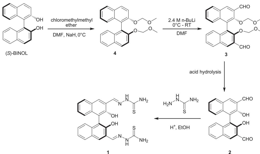
**Scheme 1.** Synthesis procedure of the sensor **1**.
