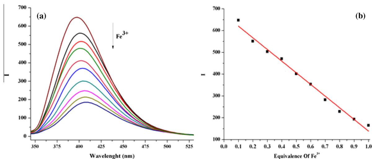
**Figure 1.** (a) Fluorescence spectra of **1** ( $1 \times 10^{-5}$  M) with an increasing concentration of  $\text{Fe(III)}$  from 0.1 to 1 equivalents (excitation wavelength = 324 nm). (b) Fluorescence decrease of **1** vs concentration of  $\text{Fe(III)}$ .
