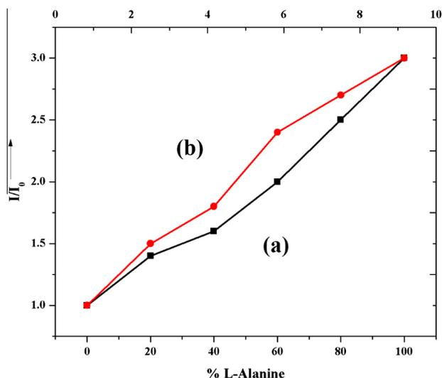
**Figure 5.** (a) Fluorescence enhancement of complex sensor ( $1 \times 10^{-6}$  mol/L) in the presence of various enantiomeric compositions of alanine. (b) Fluorescence enhancement of complex sensor ( $1 \times 10^{-6}$  mol/L) in the presence of enantiomerically pure L-alanine.
