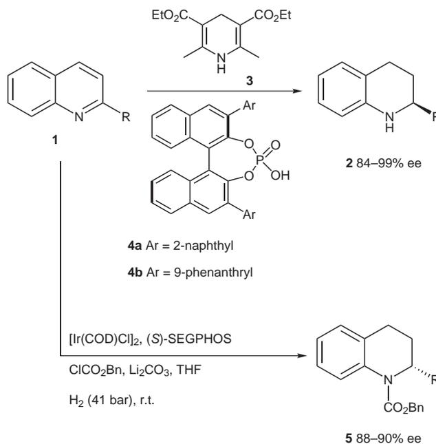
**Scheme 1** Brønsted acid and iridium-catalyzed asymmetric reduction of quinolines.
