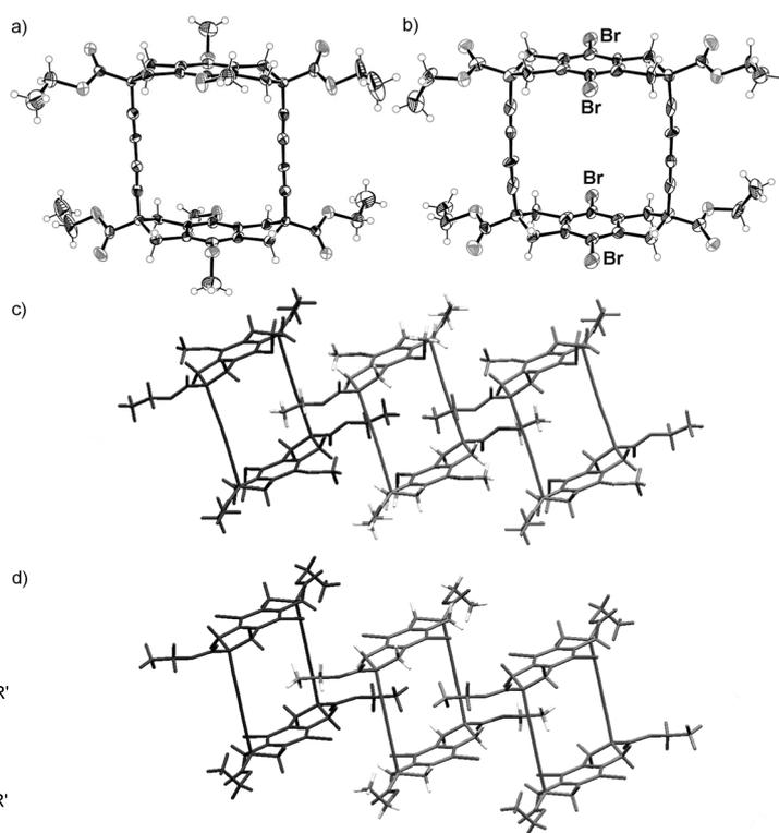
Figure 3. X-ray structures of a) **2a**-hexane solvate and b) **2b**, and c,d) their packing structures. A solvated hexane molecule in the crystal of **2a** is located outside the cavity and omitted for clarity.
