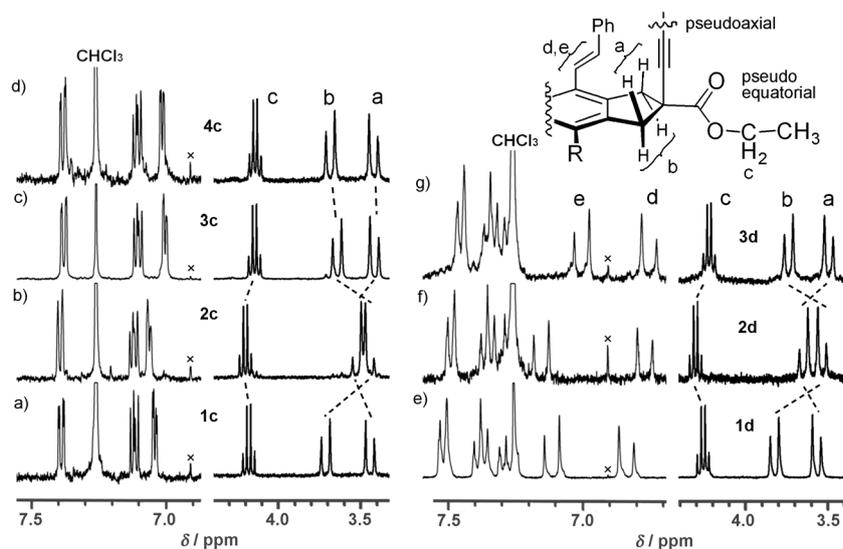
Figure 6. <sup>1</sup>H NMR spectra of a) monomer (*Z*)-**1c**; b) macrocycles **2c**, c) **3c**, and d) **4c**; e) monomer (*Z*)-**1d**; f) macrocycles **2d**; and g) **3d** in CDCl<sub>3</sub> at 295 K.
