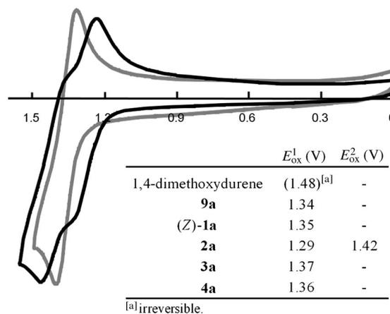
Figure 8. Cyclic voltammograms of a) **2a** (black line) and b) **3a** (gray line) measured in CH<sub>2</sub>Cl<sub>2</sub> containing 0.1 M *n*Bu<sub>4</sub>NPF<sub>6</sub> (Pt electrode, scan rate: 100 mV s<sup>−1</sup>).
