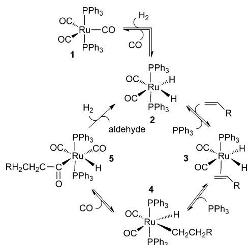
**Scheme 1.** Proposed simplified catalytic cycle of  $\text{PPh}_3$ -modified ruthenium-catalyzed hydroformylation.<sup>[45]</sup> Unsaturated 16-electron complexes have been omitted.
