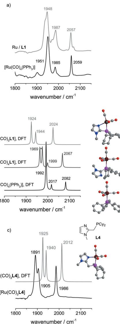
**Figure 8.** a) Comparison between experimental IR spectra for  $[\text{Ru}(\text{CO})_4(\text{PPh}_3)]$  and Ru/L1. b) Calculated vibrational spectra for  $[\text{Ru}(\text{CO})_4(\text{PPh}_3)]$ ,  $[\text{Ru}(\text{CO})_3\text{L1}]$ , and  $[\text{Ru}(\text{CO})_3(\text{L1})]$ . c) Experimental and calculated spectra for  $[\text{Ru}(\text{CO})_3\text{L4}]$ .
