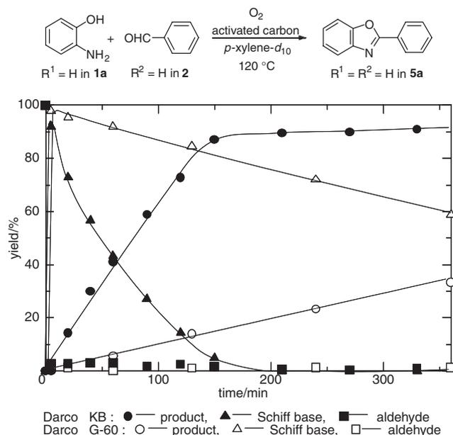
Figure 1. Time course of 2-phenylbenzoxazole, Schiff base, and aldehyde using activated carbon as catalyst. Darco<sup>®</sup> KB and G-60, which have different properties as shown in Table 2, were employed. Reactions were performed using 2-aminophenol (0.5 mmol), benzaldehyde (0.5 mmol), and activated carbon (50 mg) in *p*-xylene-*d*<sub>10</sub> (2 mL) at 120 °C under O<sub>2</sub>. Yields were determined by <sup>1</sup>H NMR analyses. Anthracene (0.1 mmol) was used as internal standard.
