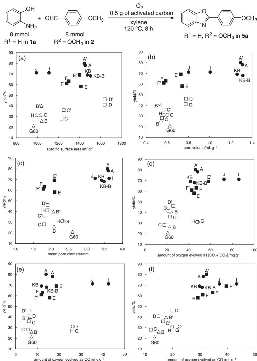
**Figure 4.** Effect of properties of activated carbons listed in Table 2 on reaction yields. (a) Specific surface area, (b) pore volume, (c) mean pore diameter, (d) amount of oxygen evolved as [CO + CO<sub>2</sub>], (e) amount of oxygen evolved as CO<sub>2</sub>, and (f) amount of oxygen evolved as CO. ●: Chemical activation (wood), ■: chemical activation (coconut shell), ○: steam activation (wood), □: steam activation (coconut shell), and △: steam activation (coal).
