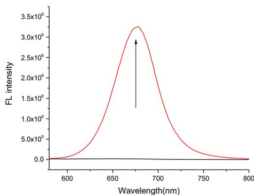
Fig. 1. (left) The UV-vis spectra of probe NR-ONOO (10.0  $\mu\text{M}$ ) in the absence (red line) and presence of  $\text{ONOO}^-$  (20 equiv.) (blue line). (right) The fluorescence emission spectra of probe NR-ONOO (10.0  $\mu\text{M}$ ) in the absence (black line) and presence of  $\text{ONOO}^-$  (20 equiv.) (red line).
