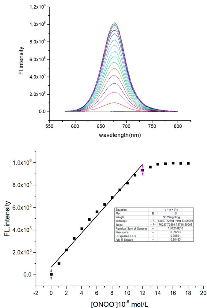
Fig. 3. (top) Fluorescence response of probe (10  $\mu\text{M}$ ) to various concentrations of  $\text{ONOO}^-$  (reaction time is 1 h) (down) Linear correlation between the enhancement of emission intensity at 638 nm.  $\lambda_{\text{ex}} = 560$  nm,  $\lambda_{\text{em}} = 678$  nm.
