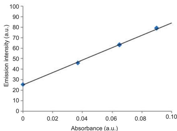
**Figure 2** Graph of emission intensity vs. absorbance of compound 5c for gradient calculation.
