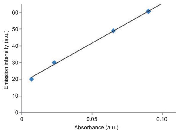
**Figure 1** Graph of emission intensity vs. absorbance of standard anthracene for gradient calculation.
