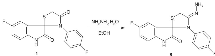
Scheme 6. Condensation reaction of compound **1** with hydrazine hydrate.
