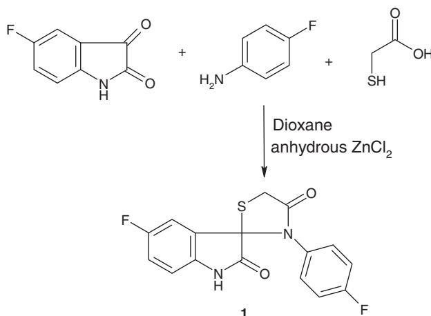
Scheme 1. The reaction of 5-fluoroisatin, 4-fluoroaniline and thioglycolic acid in the presence of anhydrous zinc chloride.
