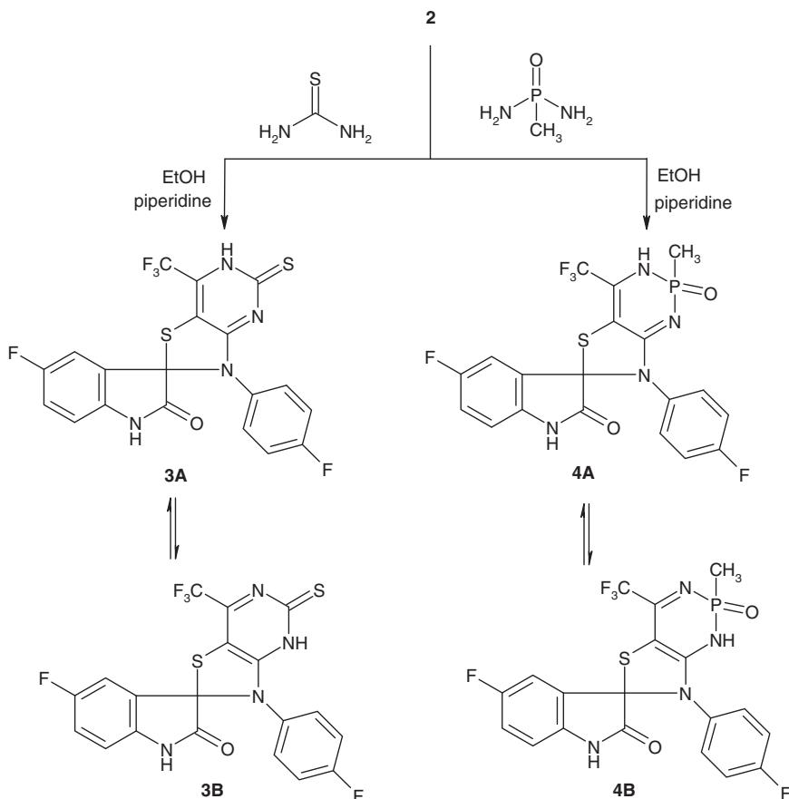
Scheme 3. The reaction of compound **2** with thiourea and methyl phosphoric diamide.
