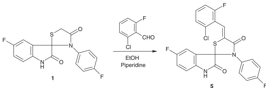
Scheme 4. Condensation reaction of compound **1** with 2-chloro-6-fluorobenzaldehyde.
