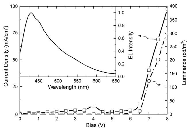
**Figure 3.**  $I$ – $V$ – $L$  characteristics of an ITO/PEDOT:PSS/**G2**/tpbi(10 nm)/CsF/Al device. Inset: normalized electroluminescence (EL) spectrum at 8 V bias.
