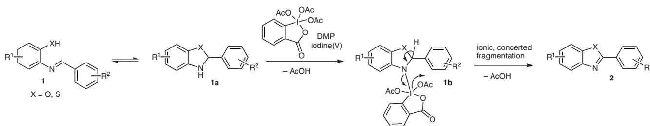
**Scheme 3** A plausible mechanism for the oxidative cyclization of azomethines mediated by Dess–Martin periodinane
