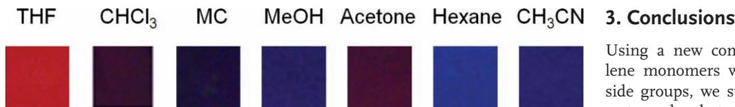
**Figure 8.** Photographs of the PDA network films after exposure to various organic solvents for 30 s.
