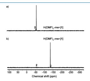
Figure 6.  ${}^{31}P{}^{1}H$  NMR (162 MHz, 25 °C) spectra of (a) reaction mixture of H(DMF)<sub>n</sub>-mer-[1] recorded after 2 days and (b) reaction mixture of H(DMF)<sub>n</sub>-mer-[1] recorded after ca. 4 weeks. 2 is phosphorane P(C<sub>6</sub>H<sub>4</sub>CO<sub>2</sub>)<sub>2</sub>(C<sub>6</sub>H<sub>4</sub>COOH).
