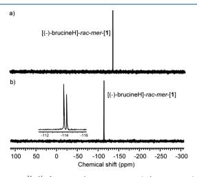
Figure 3.  ${}^{31}P{}^{1}H$  NMR (162 MHz, 25 °C) spectra of (a) [(-)-brucineH]-*rac-mer*-[1] recorded in (CD<sub>3</sub>)<sub>2</sub>SO and (b) [(-)-brucineH]-*rac-mer*-[1] recorded in CD<sub>2</sub>Cl<sub>2</sub> solvent.
