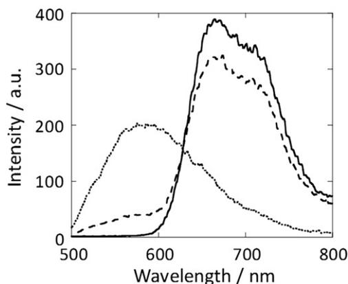
Fig. 3. Emission spectral change of **3** in hexane ( $1.8 \times 10^{-5}$  M,  $\lambda_{\text{ex}} = 420$  nm): open-form **3a** (dotted line), closed-form **3b** (solid line) and emission at photo-stationary state under irradiation with 313 nm light (dashed line).
