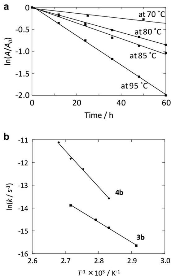
Fig. 6. Decay lines of peak absorbance by thermal cycloreversion reactions of **3b** at various temperatures (a), and temperature dependence of the thermal fading rates of **3b** and **4b** (b) in toluene.
