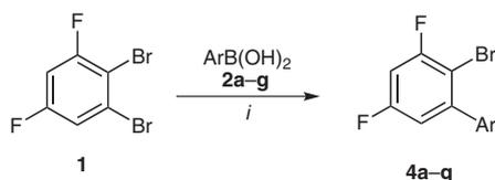
**Scheme 2** Synthesis of **4a–g**. Reagents and conditions: *i*, **1** (1.0 equiv), **4a–g** (1.0 equiv), Cs<sub>2</sub>CO<sub>3</sub> (1.5 equiv), Pd(PPh<sub>3</sub>)<sub>4</sub> (3 mol%), 1,4-dioxane, 90 °C, 9 h.
