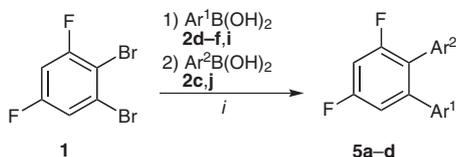
**Scheme 3** One-pot synthesis of **5a–d**. Reagents and conditions: 1) **1** (1.0 equiv), **2d–f,i** (1.0 equiv), Cs<sub>2</sub>CO<sub>3</sub> (1.5 equiv), Pd(PPh<sub>3</sub>)<sub>4</sub> (3 mol%), 1,4-dioxane, 90 °C, 8 h; 2) **2c,j** (1.2 equiv), Cs<sub>2</sub>CO<sub>3</sub> (1.5 equiv), 90 °C, 8 h.
