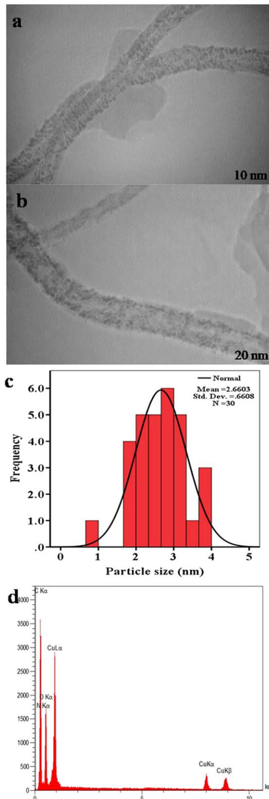
FIGURE 1 (a, b) TEM images of Cu(II)-PANi-MWCNT catalyst. (c) Particle size distribution of catalyst. (d) EDX spectrum of catalyst
