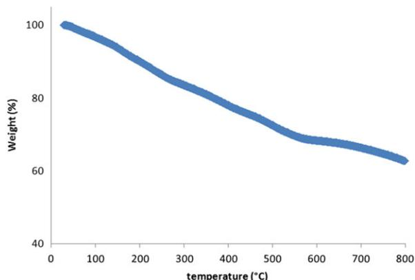
FIGURE 3 TGA curve of Cu(II)-PANi-MWCNT catalyst
