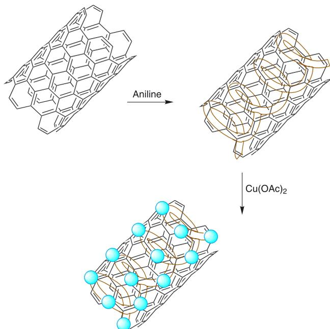
SCHEME 1 Preparation of heterogeneous catalyst Cu(II)-PANi-MWCNT
