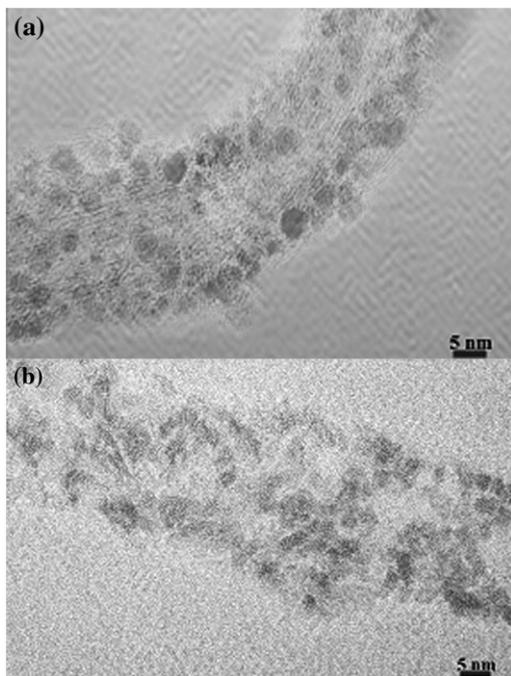
FIGURE 2 TEM images of catalyst (a) after first run and (b) after sixth run
