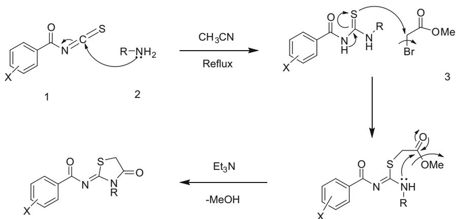
**Scheme 1** Proposed mechanism for the formation of (4-oxothiazolidine-2-ylidene)benzamide derivatives
