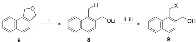
Scheme 3. Reagents and conditions: (i) Li excess (10 equiv), DTBB (5 mol %), THF,  $-78$  to  $-50$  °C; (ii) E=H<sub>2</sub>O, <sup>t</sup>BuCHO, PhCHO, Me<sub>2</sub>CO, Et<sub>2</sub>CO, (*n*-C<sub>5</sub>H<sub>11</sub>)<sub>2</sub>CO, (CH<sub>2</sub>)<sub>5</sub>CO, (EtO)<sub>2</sub>CO,  $-78$  °C; (iii) H<sub>2</sub>O,  $-78$  °C to rt.
