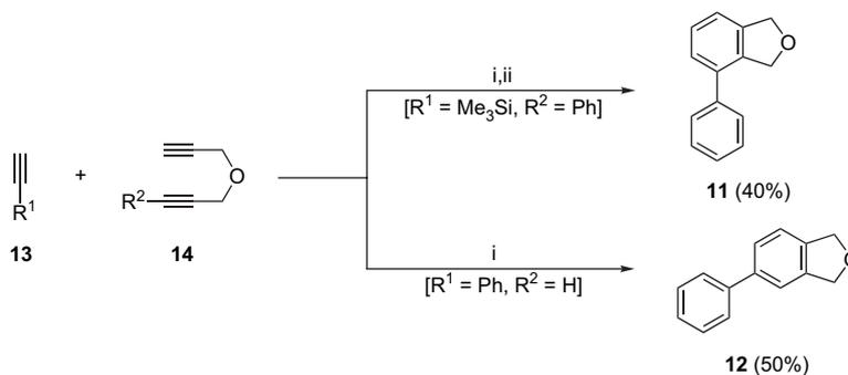
Scheme 5. Reagents and conditions: (i) Rh(PPh<sub>3</sub>)<sub>3</sub>Cl cat., PhMe, 60 (for **11**) or 0 °C (for **12**); (ii) TFA, CH<sub>2</sub>Cl<sub>2</sub>, rt.
