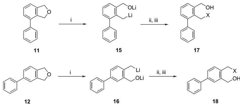
Scheme 6. Reagents and conditions: (i)–(iii) as in Scheme 3 but performing the step (i) at –78 °C.
