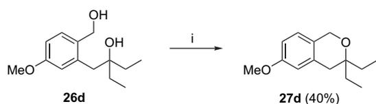
Scheme 9. Reagents and conditions: (i) MsCl, Et<sub>3</sub>N, CH<sub>2</sub>Cl<sub>2</sub>, 0 °C to rt.
