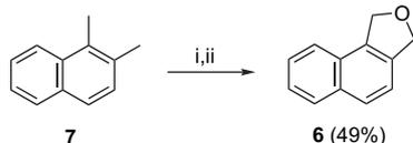
Scheme 2. Reagents and conditions: (i) 2.2 equiv NBS, AIBN cat., CHCl<sub>3</sub> reflux; (ii) 5 M NaOH, 2,6-lutidine cat., dioxane reflux.
