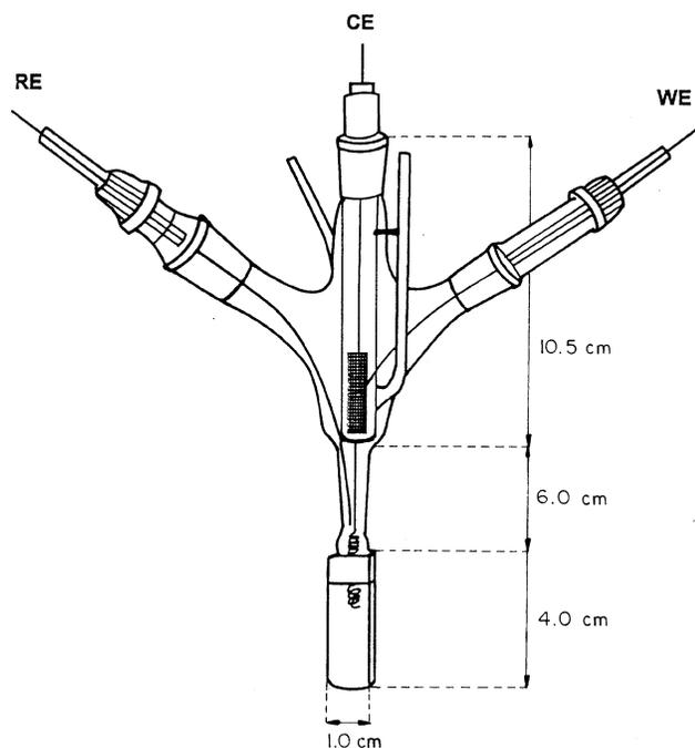
**Fig. 1** The apparatus used for measuring the *in situ* spectral changes during the constant potential electrolysis at room temperature; RE: Ag-wire reference electrode; CE: Pt-sieve counter electrode; WE: Pt-wire working electrode.
