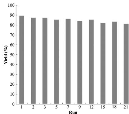
Fig. 1 Recyclability of the fiber-supported NHC catalysts for nucleophilic acylation.
