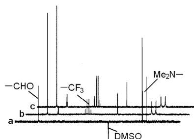
**Figure 2.** Changes in <sup>13</sup>C NMR spectra of (a) DMF, (b) DMF+TFAA (1:1) and (c) DMF+TFAA (1:2) in CDCl<sub>3</sub> at room temperature.
