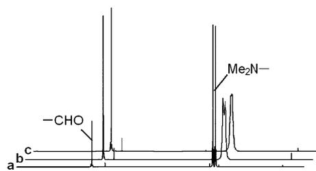
**Figure 1.** Changes in <sup>1</sup>H NMR spectra of (a) DMF, (b) DMF+TFAA (1:1) and (c) DMF+TFAA (1:2) in CDCl<sub>3</sub> at room temperature.
