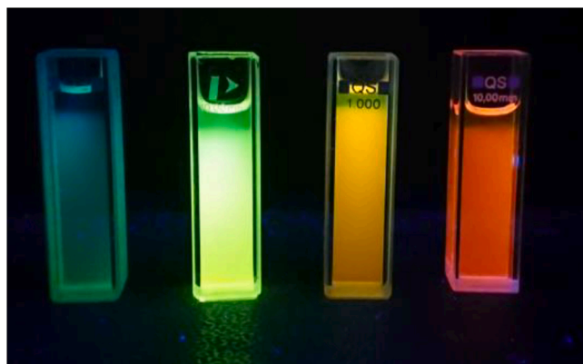
Fig. 3. n -heptane solution under UV lamp irradiation (from left to right: 7b , 8b , 7a , 8a ) c = 1\text{--}3 \times 10^{-5} M. Photographs were taken in the dark upon irradiation with a hand-held lamp ( \lambda_{em} = 366 nm).
