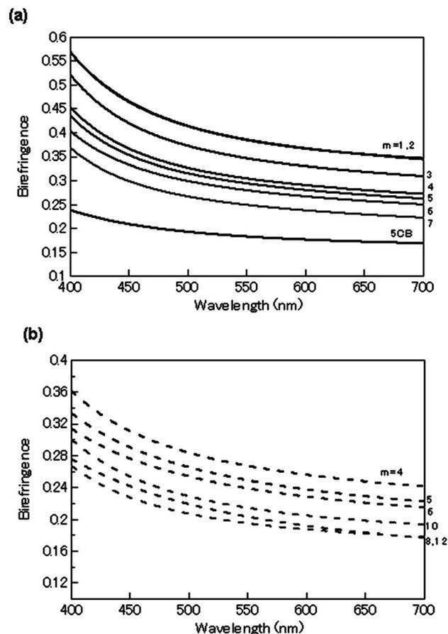
Fig. 4 Birefringence dispersion in the (a) DPDA-OC $m$  and (b) DPDA-C $m$  series. The birefringence measurements were performed at temperatures  $10^\circ\text{C}$  below  $T_i$ .
