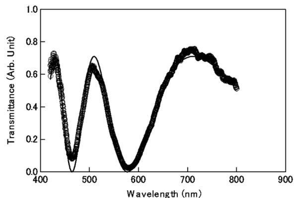
Fig. 3 Wavelength dependence of light intensity (open circles) transmitted through a homogeneous nematic cell of DPDA-OC1 under cross-polarization conditions. Here, the orientation direction of the nematic phase was set at  $45^\circ$  to the polarization axis. The solid curve is the fitting of eqn (1).
