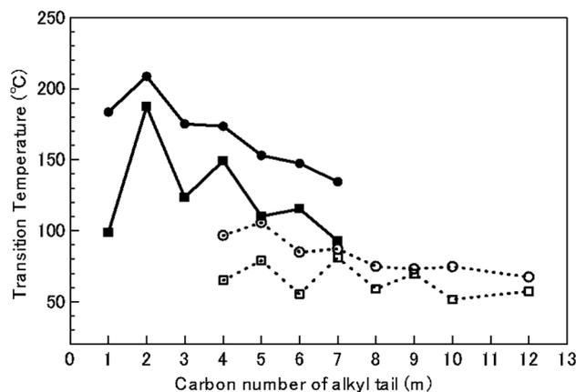
**Fig. 1** Transition temperatures plotted as a function of the carbon number  $m$  of the alkyl tail in DPDA-OC $m$  (closed symbols) and DPDA- $C_m$  (open symbols). The circles and squares are  $T_i$  and  $T_c$ , respectively.
