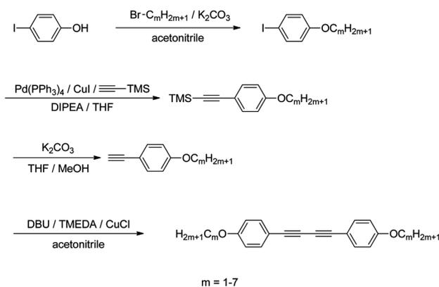
**Scheme 1** Synthesis of dialkoxy-diphenyldiacetylene (DPDA-OC $m$ ).
