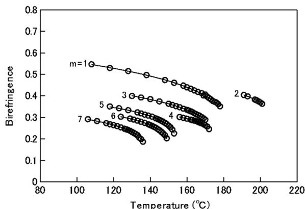
**Fig. 5** Temperature dependence of birefringence (open circles) measured at a wavelength of 550 nm for DPDA-OC $m$ . The solid curves are the fittings of eqn (5).
