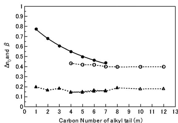
**Fig. 6** Plot of  $\Delta n_0$  (circles) and  $\beta$  (triangles) from eqn (6) determined by fitting against the carbon number  $m$  of the alkyl tail in DPDA-OC $m$  and DPDA- $C_m$ . The solid curve for the values of  $\Delta n_0$  in DPDA-OC $m$  is the fitting of eqn (6).
