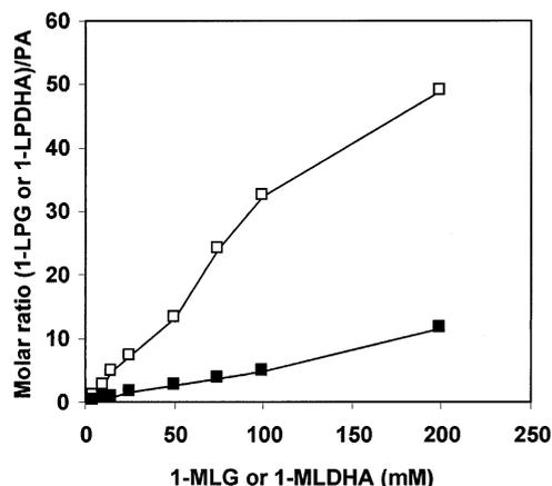
Fig. 4. Nucleophile concentration effect on the molar ratio of the transphosphatidylation and hydrolysis products. Reaction conditions containing 10 mM PC and different concentrations of 1-MLG (□) or 1-MLDHA (■) on 0.4 ml diethylether, 0.4 ml Na-acetate buffer (0.2M), pH 5.5, 40 mM CaCl<sub>2</sub> and 0.1 units PL D. Reaction temperature 25°C.
