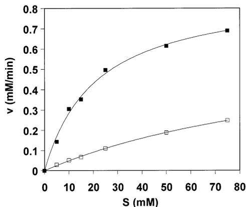
Fig. 3. Substrate effect on the initial rates for the PL D catalysed transphosphatidylation of PC (10 mM) with different concentrations of 1-monolauroyl-*rac*-glycerol (■) and 1-monolauroyl-dihydroxyacetone (□) in a diethyl ether-Na-acetate buffer (0.2M), pH 5.5, 40 mM CaCl<sub>2</sub> and 0.1 units PL D. Reaction temperature 25°C.
