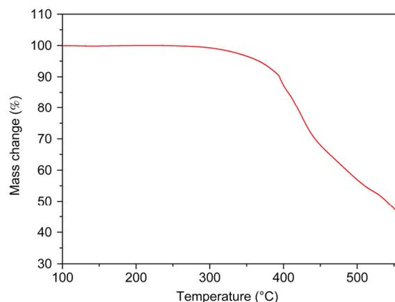
**Figure 1** TGA curve of Eu(DBM)<sub>3</sub>(BrDPPz) at a heating rate of 10 °C/min under nitrogen atmosphere.
