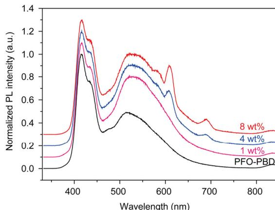
**Figure 3** Normalized PL spectra of a PFO-PBD blend and  $\text{Eu}(\text{DBM})_3(\text{BrDPPz})$ -doped PFO-PBD blend films with different dopant concentrations from 1 wt% to 8 wt%.
