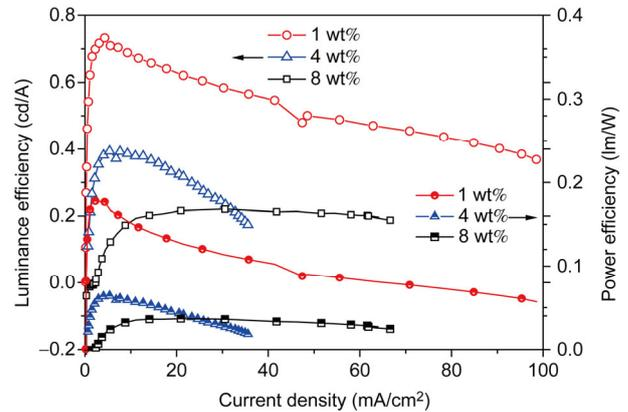
**Figure 6** Luminance efficiency-current density-power efficiency characteristics of the Eu(DBM)<sub>3</sub>(BrDPPz)-doped PFO-PBD devices with different dopant concentrations.
