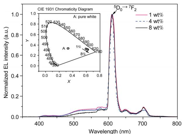
**Figure 4** Normalized EL spectra of  $\text{Eu}(\text{DBM})_3(\text{BrDPPz})$ -doped PLEDs at different dopant concentrations from 1 wt% to 8 wt%. The inset is CIE 1931 chromaticity diagrams.
