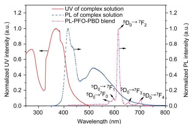
**Figure 2** Normalized UV-Vis absorption spectrum and PL spectrum ( $\lambda_{\text{ex}}=349$  nm) of Eu(DBM)<sub>3</sub>(BrDPPz) in dilute CHCl<sub>3</sub> solution and PL spectra in solution and a thin film of the PFO-PBD blend.
