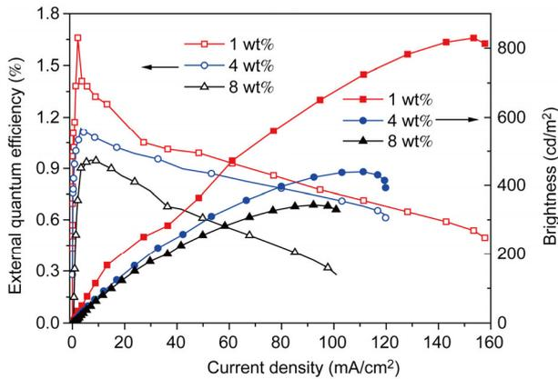
**Figure 5** External quantum efficiency-current density (EQE-*J*) and brightness-current density (*B*-*J*) curves for the Eu(DBM)<sub>3</sub>(BrDPPz)-doped PFO-PBD devices with different dopant concentrations from 1 wt% to 8 wt%.
