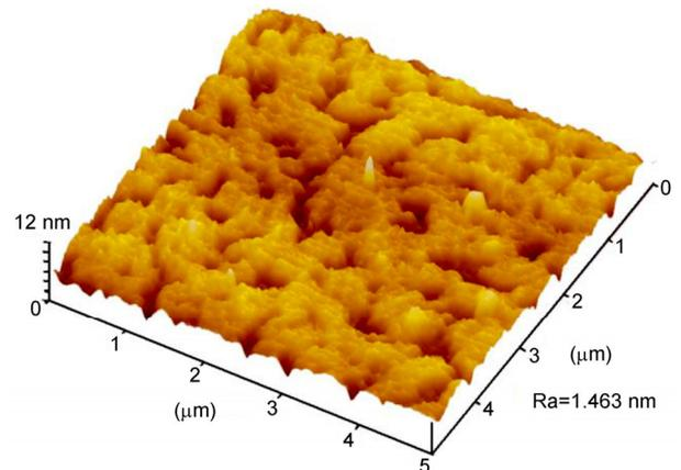
**Figure 7** Atomic force microscope (AFM) image of an Eu(DBM)<sub>3</sub>(BrDPPz)-doped PFO-PBD film containing 8 wt% dopant.
