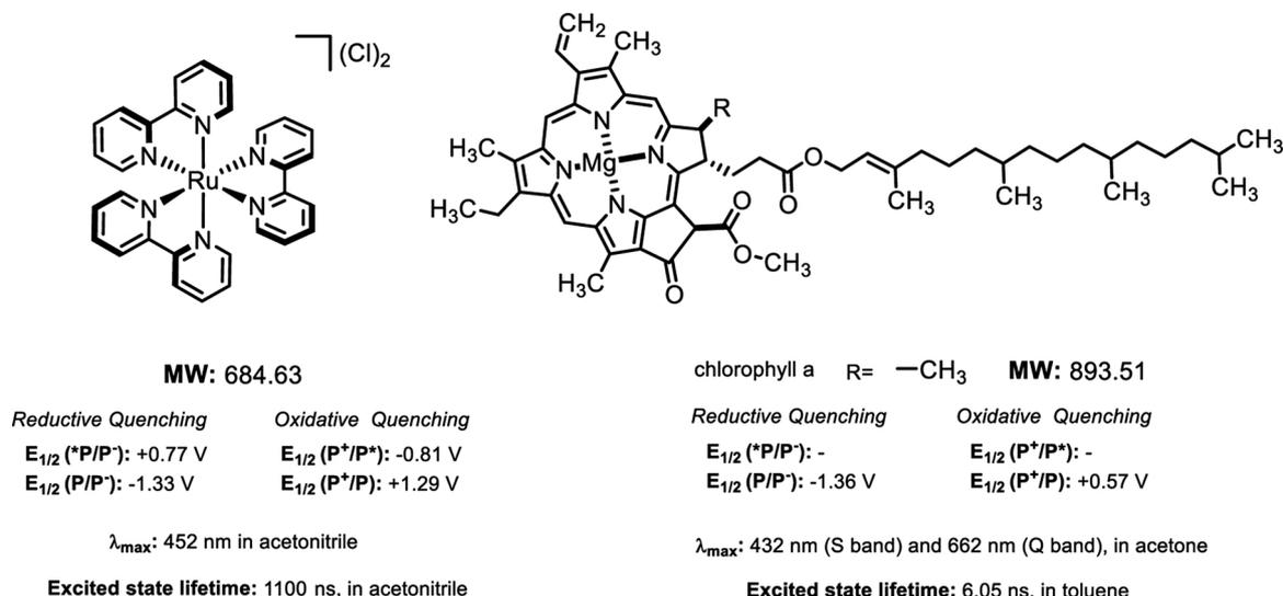
Fig. 1. Redox potentials (vs the saturated calomel electrode in acetonitrile) and selected photophysical properties of [Ru(bpy)<sub>3</sub>](Cl)<sub>2</sub> [3] and chlorophyll-a [14–16].
