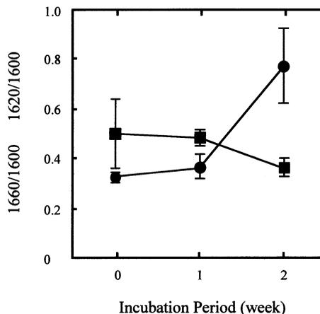
Fig. 6. Time course of the change in Raman intensity ratio during wood decay process. 1660/1600 cm<sup>-1</sup> indicates the decrease of  $\alpha$ ,  $\beta$  unsaturated bond (■) and 1620/1600 cm<sup>-1</sup> indicates the increase of carbonyl contents (●) in wood sample (*C. japonica*) during fungal decay by *C. versicolor*.
