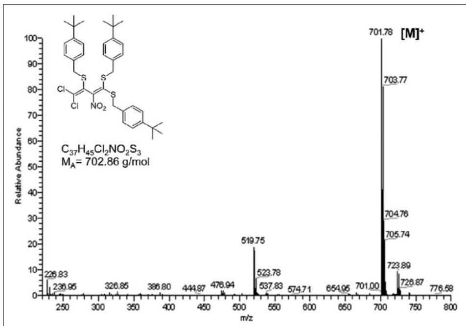
**Figure 1** Full-MS spectrum of compound **4a** in the positive mode of ESI.
