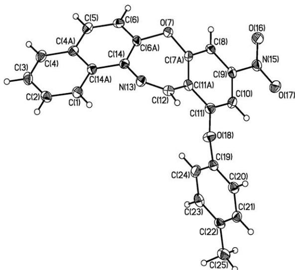
**Figure 3.** The general view of compound **4b** in representation of atoms via thermal ellipsoids ( $p=50\%$ ).
