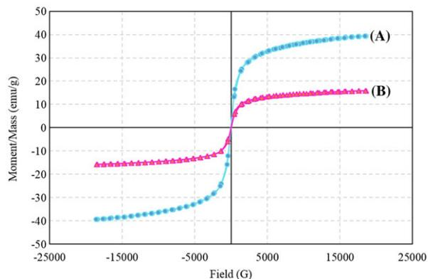
**FIGURE 5** VSM pattern of  $\text{Fe}_3\text{O}_4@SiO_2$ -MNPs (a) and  $\text{Fe}_3\text{O}_4@SiO_2$ -ZrCl<sub>2</sub>-MNPs (b)
