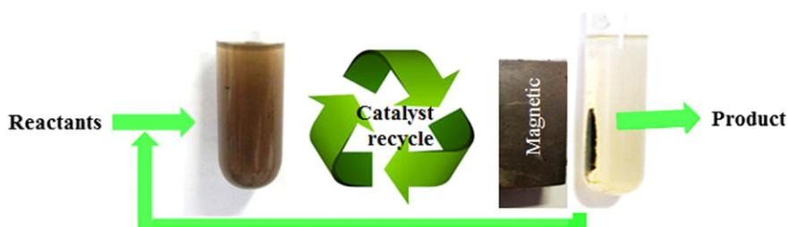
**FIGURE 6** Magnetic separation and reuse
