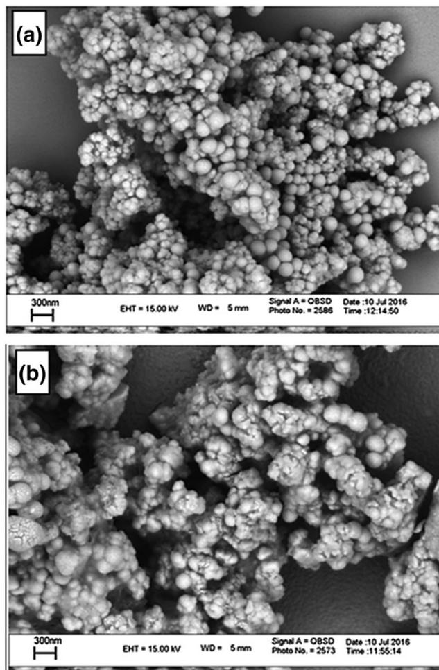
**FIGURE 3** SEM images of (a)  $\text{Fe}_3\text{O}_4@$  $\text{SiO}_2$ -MNPs (b)  $\text{Fe}_3\text{O}_4@$  $\text{SiO}_2$ - $\text{ZrCl}_2$ -MNPs
