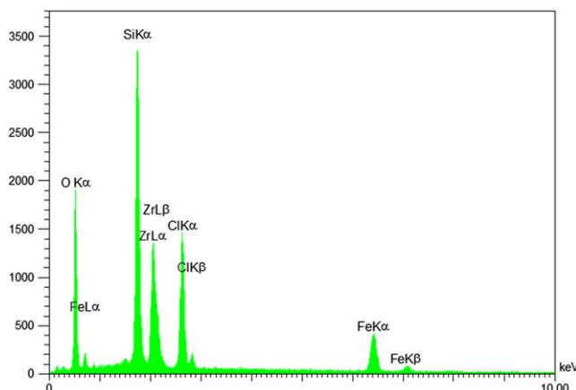
**FIGURE 2** EDX data for  $\text{Fe}_3\text{O}_4@$  $\text{SiO}_2$ - $\text{ZrCl}_2$ -MNPs
