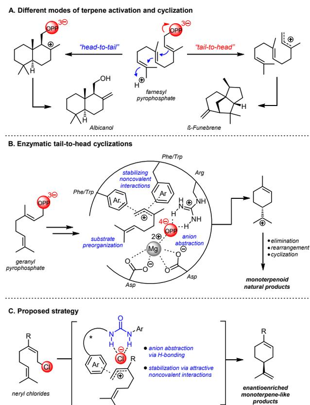
**Figure 1.** A) Head-to-tail and tail-to-head cyclization reactions. B) Schematic illustrating Nature's strategy for controlled ionization-dependent cyclizations. C) Proposed
