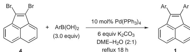
Scheme 1 Synthesis of **1** via Suzuki–Miyaura coupling.
