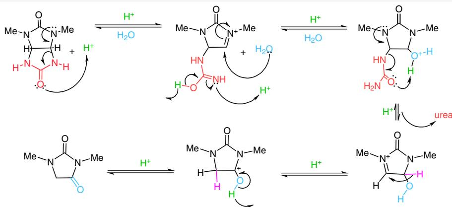
**Scheme 2** A possible mechanism of 2,4-dimethylglycoluril decomposition in acidic medium
