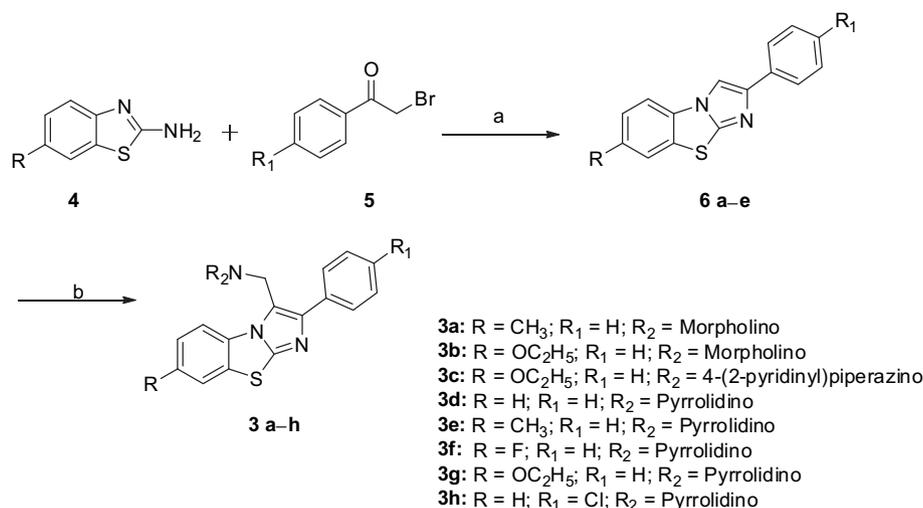
**Scheme 1.** Reagents and conditions: (a) Ethanol, MW, 180 W, 4–5 Min, 77–82%; (b) ZnCl<sub>2</sub>, secondary amine, HCHO, Ethanol, 4–5 h, rt, 84–91%.
