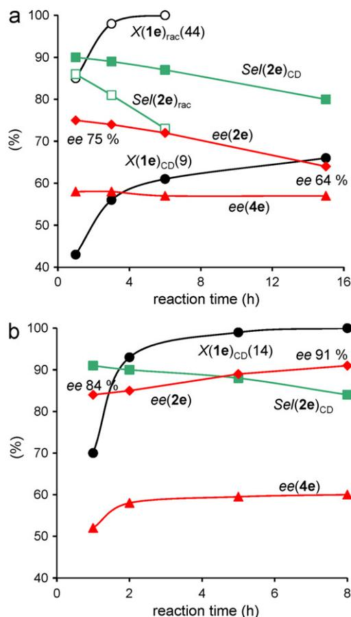
**Fig. 3.** Hydrogenation of **1e** over unmodified and CD-modified catalyst in the absence (a) and presence of BA (b). Reaction conditions: see Table 2. For abbreviations see Figs. 1 and 2 (the formation of **3e** was detected only over modified catalysts,  $\text{Sel}(3\text{e}) = 4\text{--}5\%$  and  $2\text{--}4\%$  in the absence and presence of BA, respectively).
