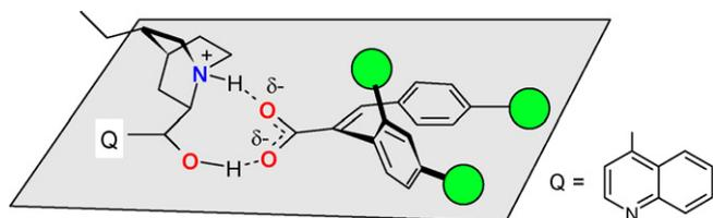
**Fig. 5.** Schematic illustration of the arrangement on the Pd surface of (*E*)-2,3-diphenylpropenoic acids interacting with the modifier.
