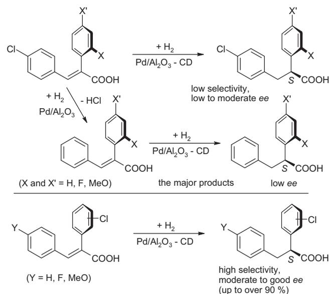
**Scheme 2.** Reaction pathways observed in the enantioselective hydrogenation of Cl substituted (*E*)-2,3-diphenylpropenoic acids over CD-modified Pd catalyst.
