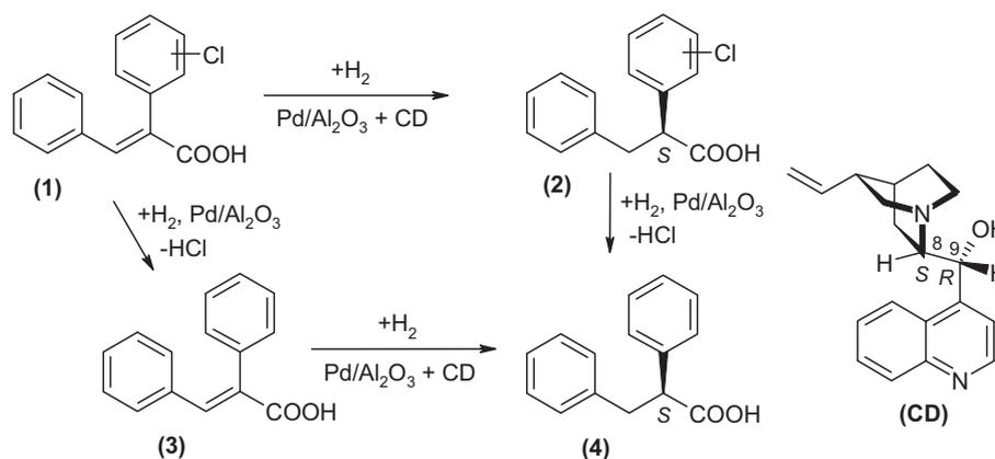
**Scheme 1.** Example of the possible reaction pathways in the enantioselective hydrogenation of Cl substituted (*E*)-2,3-diphenylpropenoic acid derivatives over CD-modified Pd catalyst.
