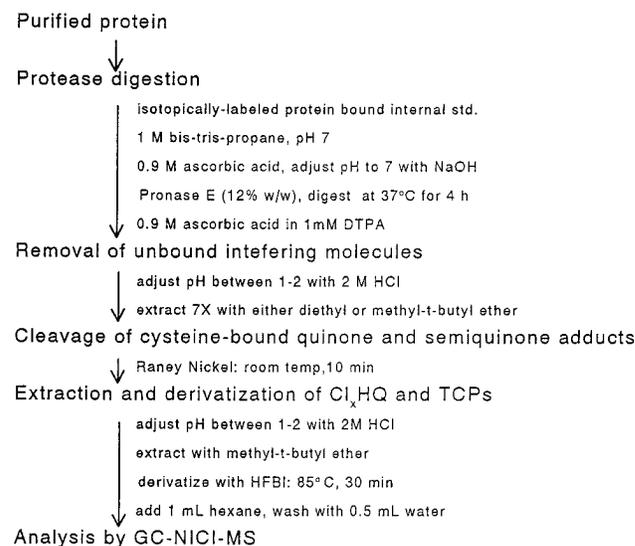
**Figure 4.** Outline of the assay to measure PCP-derived quinone and semiquinone adducts.
