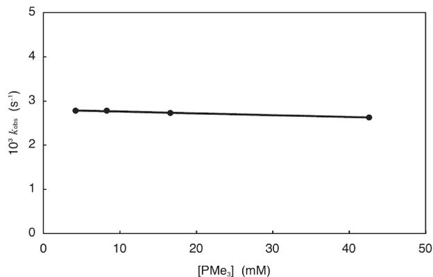
**Figure 3.** Effect of added PMe<sub>3</sub> on the first-order rate constant  $k_{\text{obs}}$  monitored by the UV–vis spectral change at 518 nm for conversion of **2d** into **1d** in benzene at  $30.0 \pm 0.5$  °C. Conditions:  $[\mathbf{2d}] = 0.94 \text{ mM}$ .
