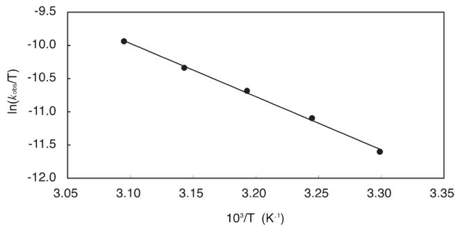
**Figure 4.** Eyring plot for the intramolecular C–H bond cleavage reaction of **2d** to give **1d** in benzene.
