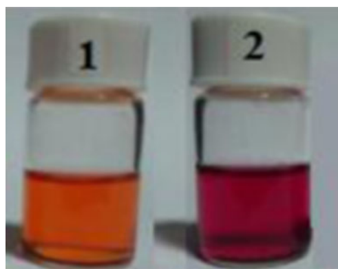
Fig. 3 The color change of the sensor upon complexation with \text{Hg}^{2+} ions (1 ATBD; 2 ATBD + \text{Hg}^{2+} )
