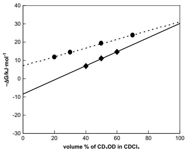
**Figure 1.** Relationship between  $-\Delta G$  of aggregation of macrocycles **1b** and **2b** and the composition of  $\text{CD}_3\text{OD}$  in  $\text{CDCl}_3$ ; solid circle: **1b** (Ref. 2f), solid square: **2b**.
