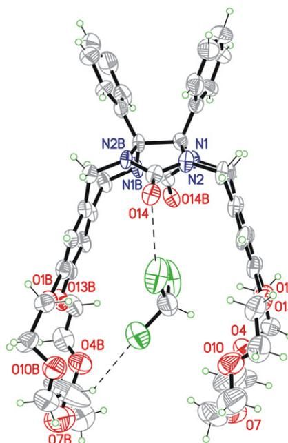
Fig. 4. ORTEP drawing of complex **2**·CHCl<sub>3</sub> with partial labeling scheme. Thermal ellipsoids are shown with the 30% probability level.
