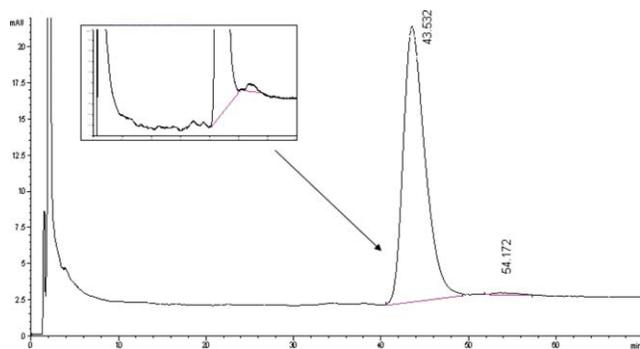
**Fig. 4.** Chromatogram of virtually enantiopure benzyl (2*S*,3*R*)-2,3-dihydroxy-3-(3,4-dibenzyloxyphenyl)-propionate. Chiral column: Sepapak-4; mobile phase: *n*-hexane/2-propanol (85/15 v/v); flow rate 2.0 ml/min. The major product is produced using the chiral auxiliary (DHQD)<sub>2</sub>-PHAL. (ee = 98.2%). [Color figure can be viewed in the online issue, which is available at [www.interscience.wiley.com](http://www.interscience.wiley.com).]
