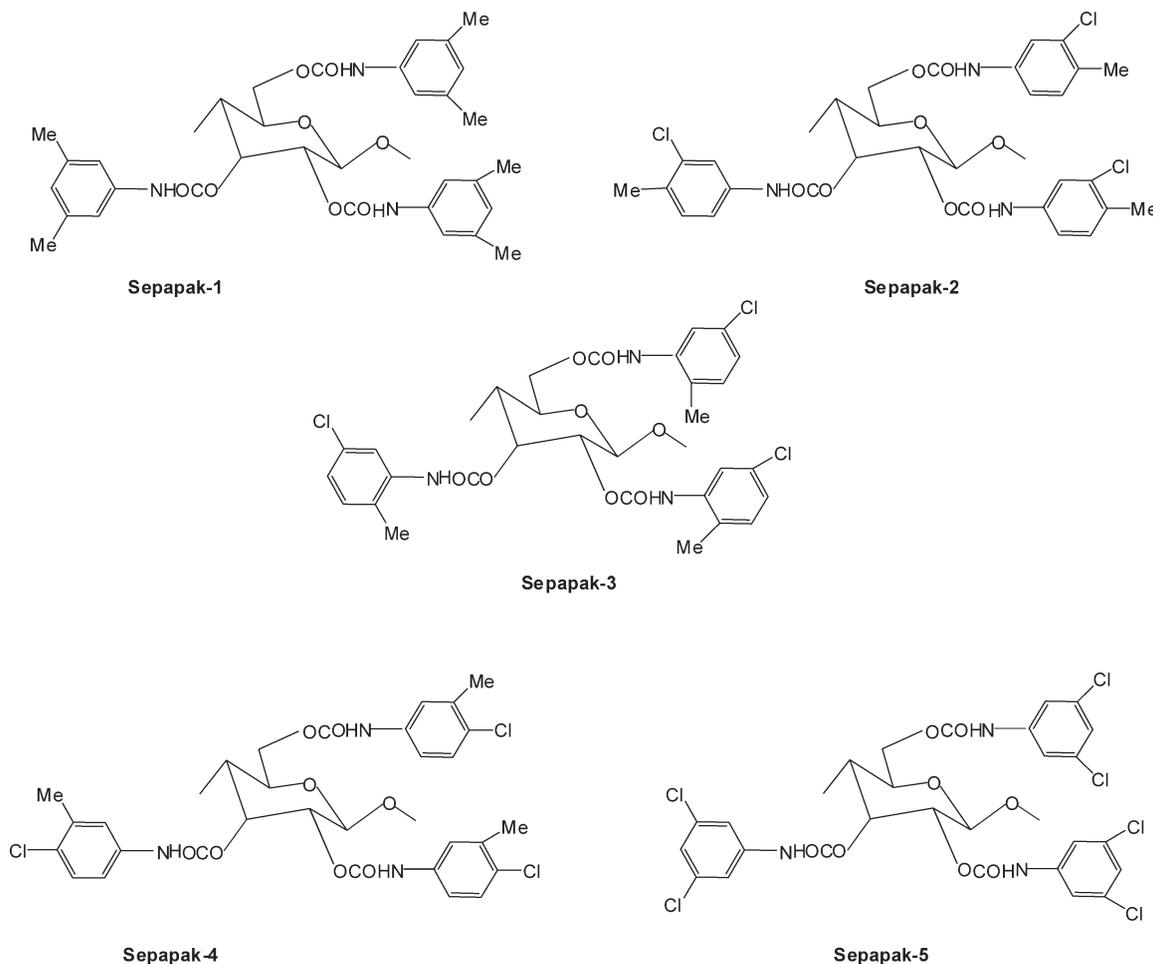
**Fig. 5.** Structures of filling materials in Sepapak columns. Sepapak-1: cellulose tris-(3,5-dimethylphenylcarbamate); Sepapak-2: cellulose tris-(3-chloro-4-methylphenylcarbamate); Sepapak-3: amylose tris-(5-chloro-2-methylphenylcarbamate); Sepapak-4: cellulose tris-(4-chloro-3-methylphenylcarbamate); Sepapak-5: cellulose tris-(3,5-dichlorophenylcarbamate).
